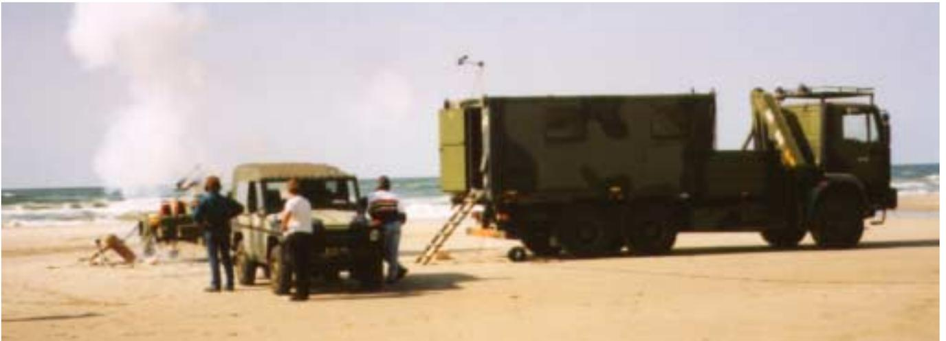
The test set up. The gun and radar is on the left with the radar behind it. The vehicle to the right contains the office and computer
