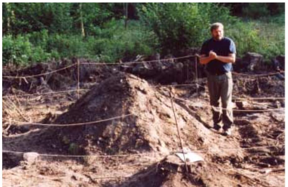
The charcoal heap after firing and ready for opening
