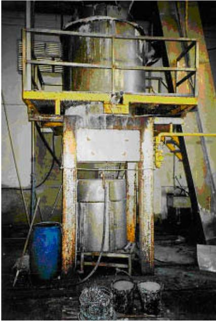
Figure 12 The iron reaction vessel
