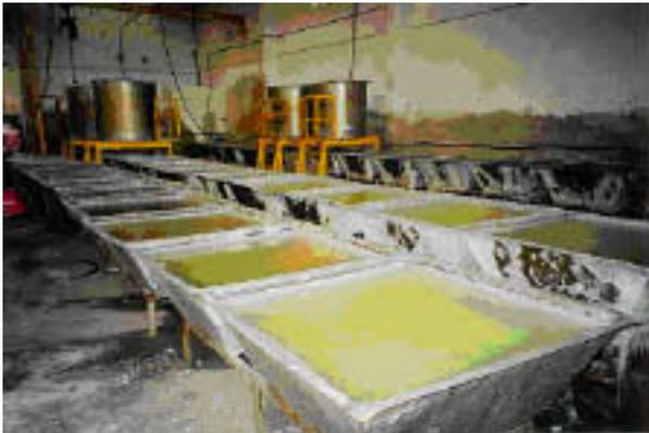
Figure 14 The crystallisation pans
