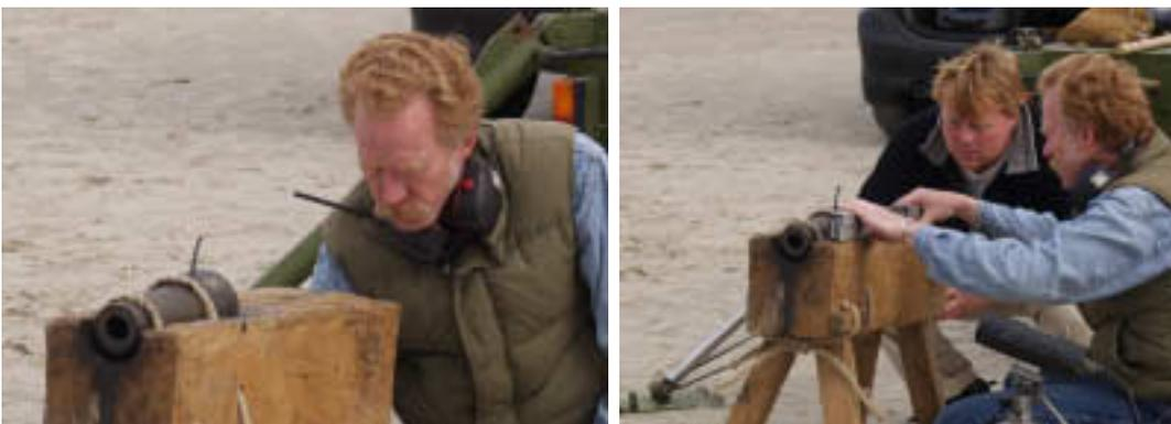
Figure 7 Left, taking aim. Right setting and measuring the elevation of the gun using a clinometer
